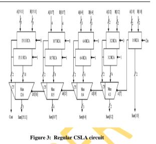
The structure of the 16-b regular SQRT CS conventional carry select adder performs better in terms of speed. The delay of our proposed design increases lightly because of logic circuit sharing sacrifices the length of parallel path.
