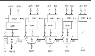
Figure 4: CSLA circuit using BEC Converter
